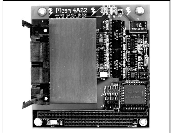
The 4A22 is low power integrating 18 bit data acquisition system for the PC/104 bus. The 4A22 has 14 input channels with 500V isolation from system ground. The analog inputs have software selectable 0.5V or 5V full scale ranges.
