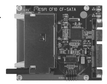
The CFADPT10 is a SATA to Compact Flash adapter on a small PCB. The form factor matches a 2.5" SATA hard drive.
