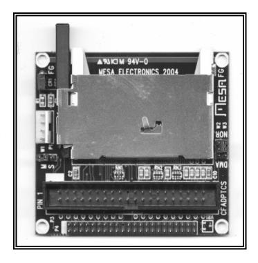
The CFADPT-CS is an small adapter to allow connecting compact flash cards to systems with IDE interfaces.
