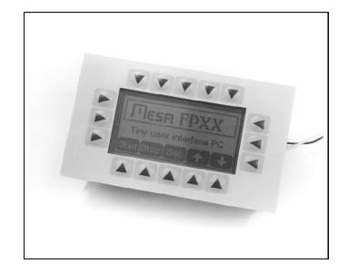
The keyswitch array surrounds the display area so that the keys can be labeled in the display. Each key can return a user selectable scan code. The FPXX BIOS provides support for soft-key graphic labels.
