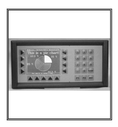
Two FIFOed serial ports are provided as is a bi-directional parallel port. One of the serial ports can be configured for RS-485 interface levels. A 1.44M floppy and IDE interface allow external storage if needed.
