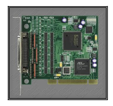
The 5I21 is suitable for high performance motion control systems, Robotics, Industrial I/O, Custom real time distributed I/O, time code generation, supporting legacy hardware, and almost any high speed serial interface application that requires a flexible, high performance, universal RS422/485 serial interface card.
